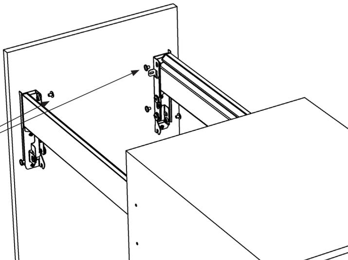
2. Tilt the door panel forward till the door bracket is clear of the top adjustment cam.
